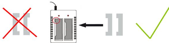
Connect the main adaptor to the charger and turn the power on. Control indicators will begin to blink. The charging process can take up to 18 hours to complete.
