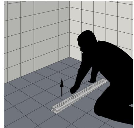
2. Remove the grating plastic locks from the sides of the grating and insert the LED unit making sure that the LEDs are facing toward the center of the grating while the angled top faces upward allowing water to drain freely.
