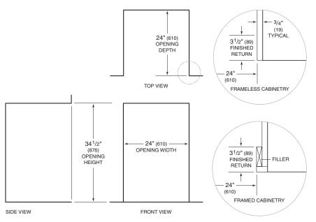
NOTE:  $3^{1}/2^{\circ\prime\prime}$  (89) finished returns will be visible and should be finished to match cabinetry.
