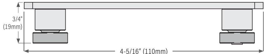
Ball bearing double roller, stainless steel
