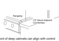
Front of deep cabinets can align with control panel beveled edge.
