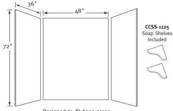
Designed to fit base areas 36" deep or smaller x 48" wide x 72" high or smaller (914 mm x 1219 mm x 1829 mm)
