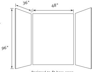
Designed to fit base areas 36" deep or smaller x 48" wide x 96" high or smaller (914 mm x 1219 mm x 2438 mm)
